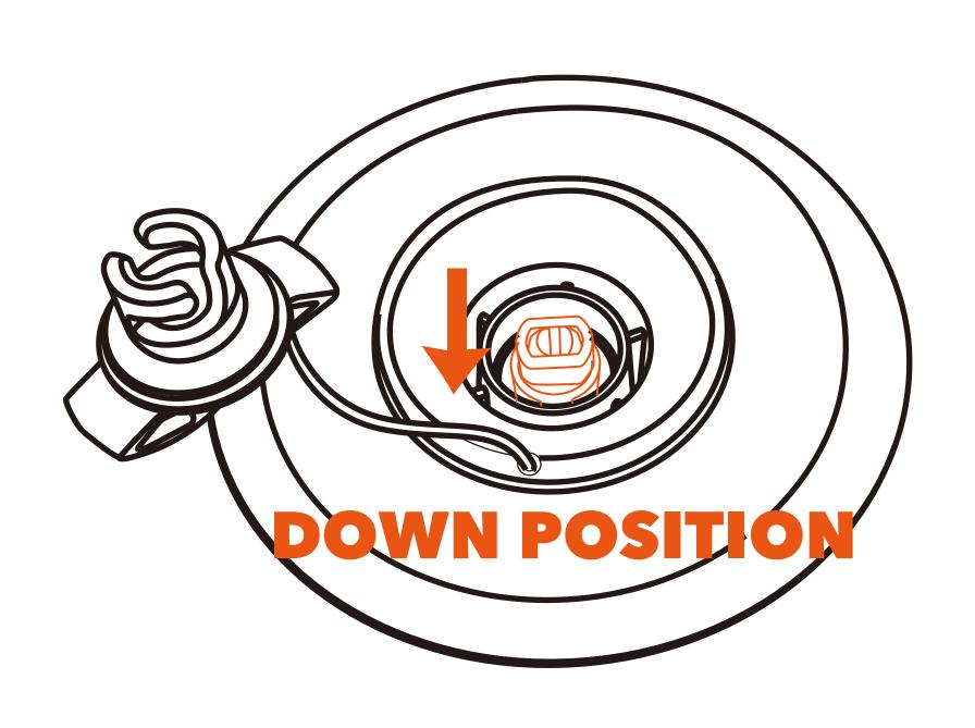
Valve button popping up to the "UP position" for inflation. Valve button locked in "DOWN position" for deflation.
