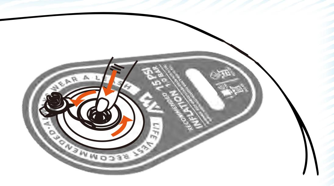
Open the valve cap by twisting counter-clockwise.
